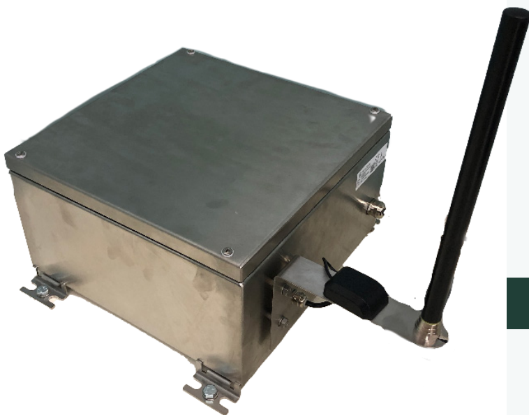
Tilia Accelerograph installed in protective field cabinet.
